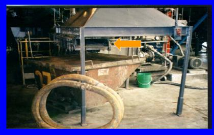
Solids from a Subpart X unit are routed out of the unit via a conveyor to a hopper. See arrow. The hopper is placed under a hood to capture some of the emissions. The existing configuration had calculated capture efficiency of less than 35%. The new configuration will reduce emissions by almost 99%.
